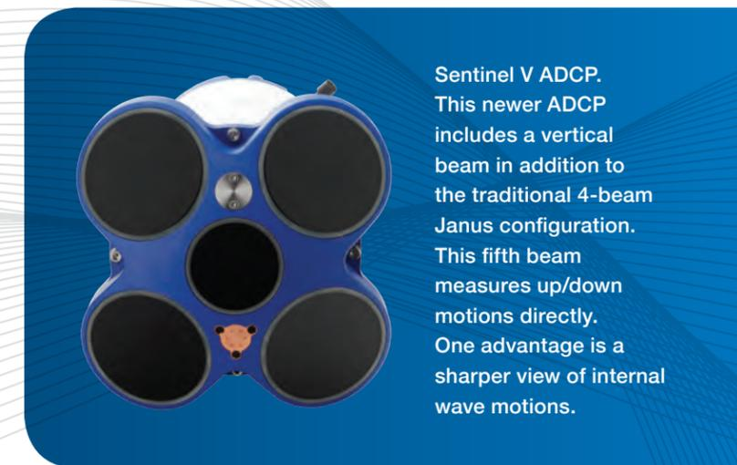
**Sentinel V ADCP.** This newer ADCP includes a vertical beam in addition to the traditional 4-beam Janus configuration. This fifth beam measures up/down motions directly. One advantage is a sharper view of internal wave motions.
