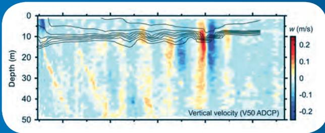
Contour view of vertical (up/down) currents along the measurement transect. Red colors indicate regions of upward flow whereas blue colors depict downward motion. To the right side of the panel are stronger motions associated with an internal solitary wave.
