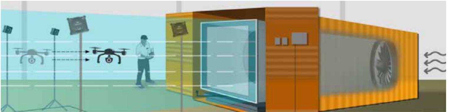
Boston Engineering received an AFWERX SBIR Phase I contract to advance its beta Wind Profile Generator™ for small Unmanned Aerial Systems (sUAS). The portable system accelerates sUAS testing and training by monitoring sUAS tests in controlled, uniform, laminar air flow. The Wind Profile Generator is the only standard/networked sUAS system that combines robust testing capabilities, scalability, and portability
