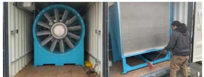
**Wind Profile Generator Portable Fan**
