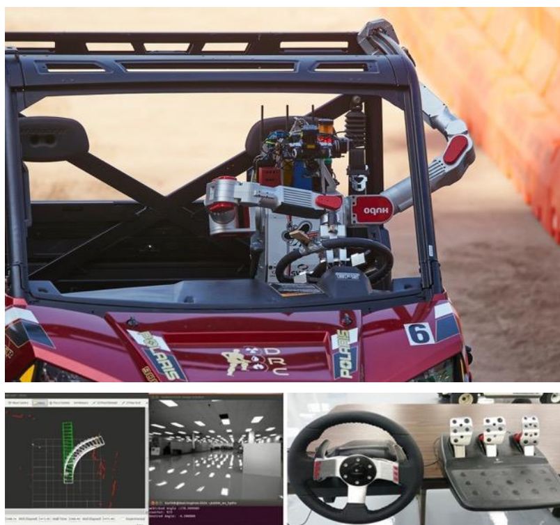
Figure 11. Team DRC-HUBO at UNLV performing the Vehicle task. Top: The robot operating the car. Photo from http://www.drc-hubo.com/ (accessed August 2017). Bottom: The operator's interaction method for driving the car, showing the car trajectory on the left and the steering wheel and foot pedal input devices on the right. Image from Oh et al. (2017).
